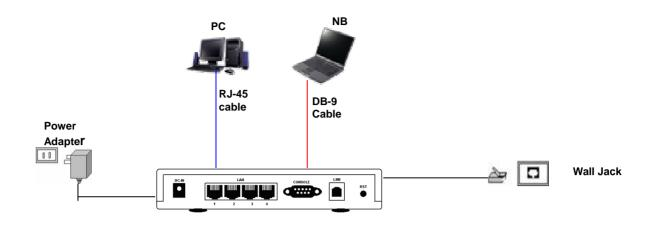
Figure 2-2 Direct Connection with PC or NB
